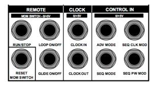
Sadly, it is possibile to make some confusion if you are using ROW C for CV generation connected at SEQ MODE input port: **R24** works correctly, but it can land on a potentially useless condition.
