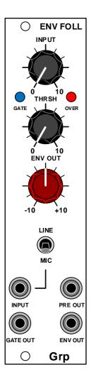
CV and Gate extraction from audio signal with Line/Mic selectable level There is a pre-amped audio signal output
